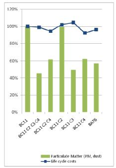
Figure 7-22: BC11: Pellet boiler - Total life cycle cost (LCC) and BAT (in terms of PM) per option
