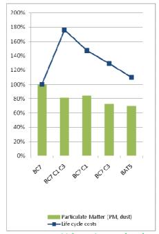
Figure 7-14: BC7: Pellet stove – Total life cycle cost (LCC) and BAT (in terms of PM) per option
