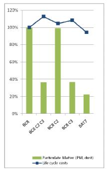
Figure 7-16: BC8: Conv. domestic boiler - Total life cycle cost (LCC) and BAT (in terms of PM) per option
