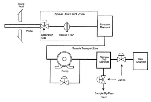
Figure 1-13: Example of the installation for measuring devices<sup>34</sup>
