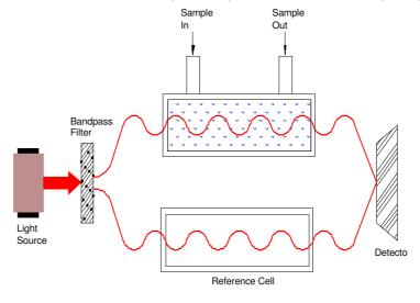
Figure 1-15: Example of a NDIR analyser<sup>36</sup>
