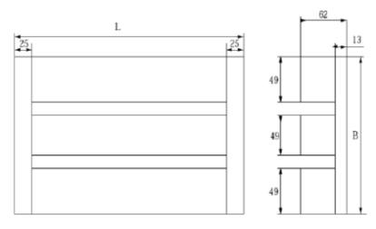
Figure 1-17: Arrangement of the standard test fuel
