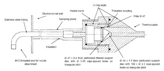
Figure 1-22: Suggested arrangement of dilution tunnel filter housing<sup>43</sup>
