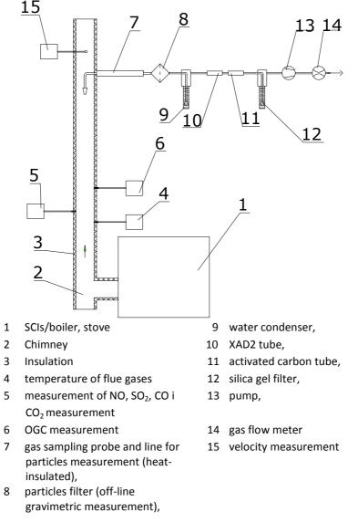
Figure 1-19: Scheme of particle (dry particle) and organic pollutants sampling direct from hot exhaust gas<sup>41</sup>
