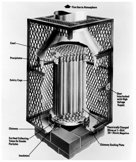
Figure 1-20: Smoke measurement by electrostatic precipitator<sup>42</sup>
