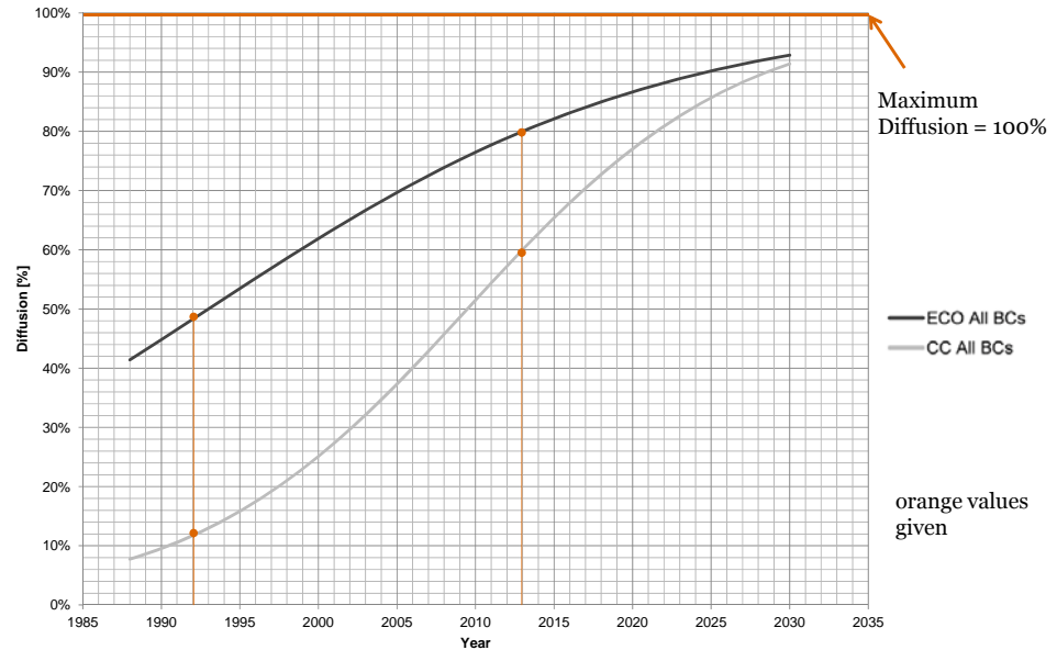
Figure 83 - Assumed s-curve for the Economizer (ECO) and Combustion Control (CC)
