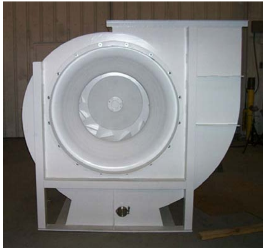
Figure 54 - Picture of a draft fan used in industrial steam boilers
