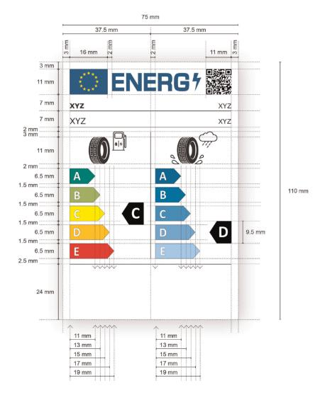
2.1.1. Format of the bottom part of the tyre label for all tyres other than tyres which satisfy the minimum snow grip index values set out in UNECE Regulation No 117, or the relevant minimum ice grip index values, or both:
