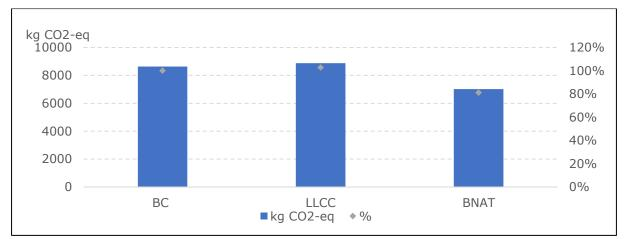
Figure 24: Emission of CO<sub>2</sub> (kg CO<sub>2</sub>-eq) of the base case, LLCC and BNAT – for BC 2 (split 7.1 kW)
