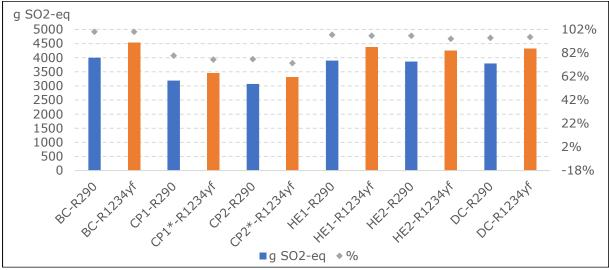
Figure 10: Emission of acidifying agents (g SO<sub>2</sub>-eq) of the base case and the different improvement options – for BC 3 (single duct 2.6 kW– R290 and R1234yf)
