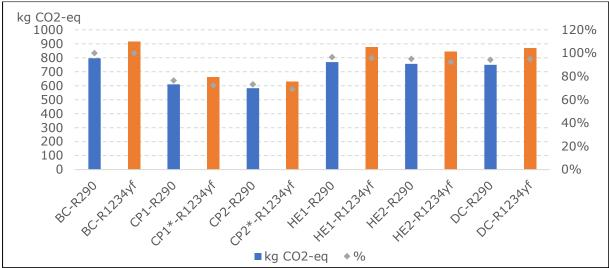
Figure 9: Emission of CO<sub>2</sub> (kg CO<sub>2</sub>-eq) of the base case and the different improvement options – for BC 3 (single duct 2.6 kW– R290 and R1234yf)
